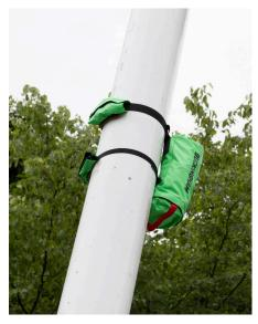
Newly designed setup allows for hurt man rescue system to be permanently attached to boom without risking damage to components because of weather. Gum rubber allows for secure placement on the boom.
