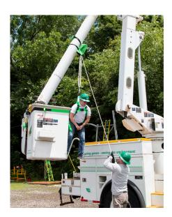
4:1 pulley system allows for easy lifting of injured worker. Photos used for demonstration purposes only. Always wear your PPE.
