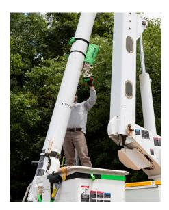
In case of rescue situation, simply tear away the cap with the red webbing and components will drop out easily and freely.
